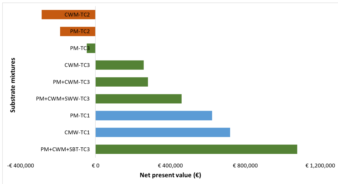
Figure 6-2: Comparison of mixtures by treatment concept. TC: treatment concept, PM: pig manure, CWM: cow manure, SWW: starch wastewater, SBT: sugar beets.
