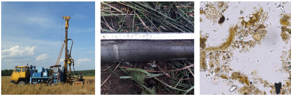
Figure 2.4: Drilling of a sediment core (left), the resulting core (center) and microscopy image data (right). (Images provided by the University of Greifswald)
