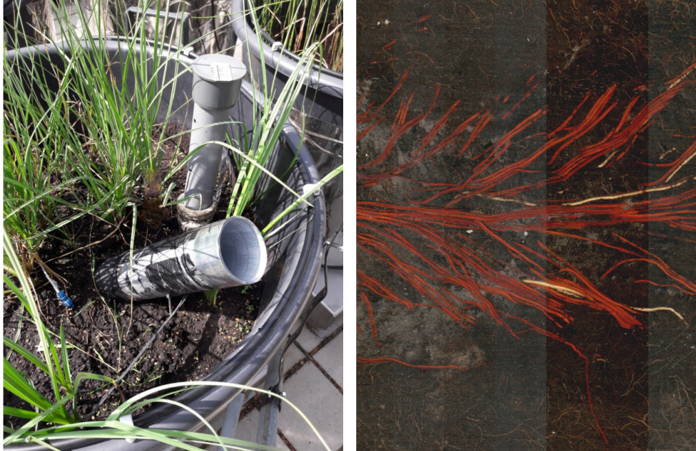
Figure 2.2: Minirhizotrons in a mesocosm experiment (left) and a crop of the resulting minirhizotron image data (right). (Images provided by the University of Greifswald, slight modifications added)
