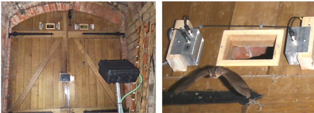
Figure 2.3: Camera trap setup triggered by infrared light barriers (left) and a crop of a typical camera trap image, recording a bat flying through the opening. (Images provided by the University of Greifswald)
