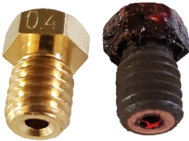
Fig. 1. FDM nozzles with different degrees of wear and clogging (which, in principle, were also used for the investigations). Left: a completely new nozzle, right: a used nozzle with over 50 h of printing time.
