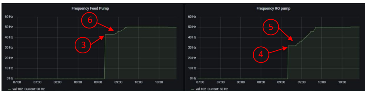
Figure 59 the control system adjusts the frequency of all pumps to optimize energy sharing and maximize water production.
