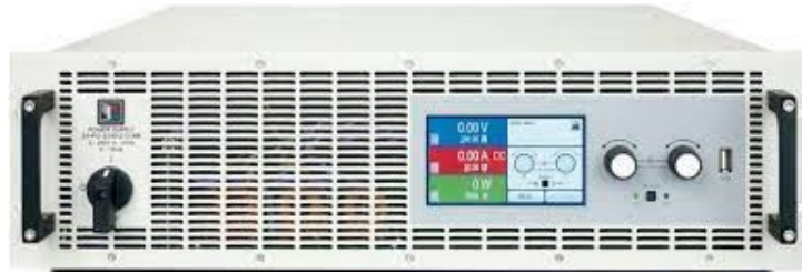
Figure 46 two DC Power suppliers from Datatec (series 9000) are used to simulate the solar power for each MPP tracker. The performance accuracy of the system is <0.1%, the Load Regulation 0-100% accuracy is <0.05%, the accuracy of the Line regulation \pm 10\% \Delta U_{AC} is <0.02%, the Regulation Speed 10-100% load is <2 ms, and Slew rate 10-90% is maximum 30 ms.
