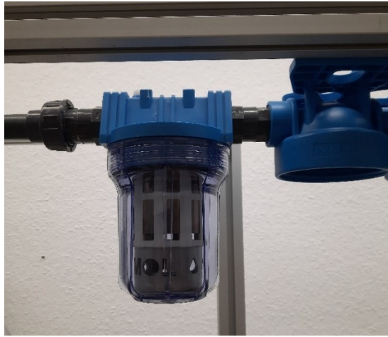
Figure 77 MOL®LIK SW30 is used to improve the pre-filtration system of the test bench.
