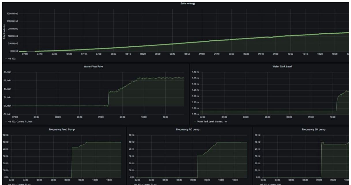
Figure 57 start-up process of the pilot project in Ghana on a typical sunny day.
