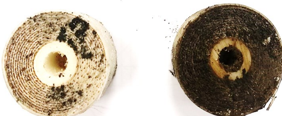
Figure 64 cut cross-section of membranes from the first stage. Left: the membrane from the test bench after four months of running, equal to 16 months of regular running. Right: the membrane from the pilot project in Cape Coast is removed from the system after twelve months of working.
