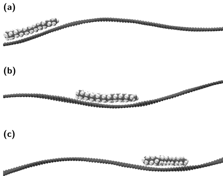
Figure 4.13: Snapshots of the NPs-1L models showcasing the diffusion of PE in the xy plane on the graphene surface, with configurations: (a) within the first 5 ns, (b) within the second 5 ns, and (c) within the last 5 ns. The water molecules are hidden for clearer visualization.
