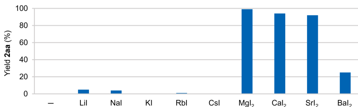
Figure 1. Screening of alkali and alkaline earth metal iodides with Et 3 N for the conversion of butylene oxide ( 1aa ) to butylene carbonate ( 2aa ). Reaction conditions: 1.0 equiv. of 1aa (10.0 mmol), 2 mol% salt MI n and 2 mol% Et 3 N, 23°C, 24 h, solvent free, p (CO 2 ) = 1 bar. Yields were determined by 1 H NMR using mesitylene as the internal standard.
