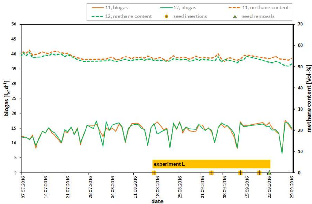
Supplementary Figure 2-4 | Biogas yield (solid lines) and methane content (dashed, thick lines) during the operation of the lab-scale reactors 11 and 12 at 42°C. Above the x-axis, it is indicated when seeds were inserted or removed from the reactors (labeled as experiment L).
