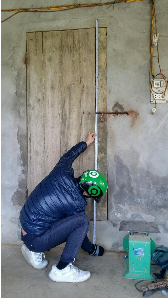
Figure 8.1. Flood mark of 2018 at Xuan Linh hamlet, Thuy Xuan Tien commune, Chuong My district (Flooding depth: 2.5 m, Lat/Long: 20.880, 105.562)
