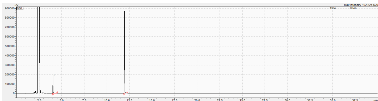
Figure 62. Exemplary gas chromatogram of dimethyl oxalate ( 87 , t_R = 4.03 min) and tetradecane (IS, t_R = 11.96 min) using a 40 min-method heating von 50 °C to 280 °C with a heating rate of 10 °C/min.
