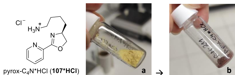
Figure 20. Pyrox-C 4 N as hydrochloride salt 107*HCl . The compound in a) was freshly prepared, while in b), it was stored under air for two weeks.
