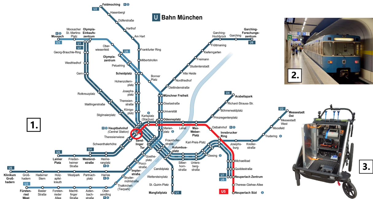
Figure 4-3: 1. Overview of the Munich subway system [93], with the studied area marked in red and the sampling location for automated SEM/EDX imaging encircled 2. Sampling location for testing of the automated imaging algorithm [94] 3. Mobile measurements system for online analysis and offline sampling. Adopted and modified from Neukirchen et al. [65]
