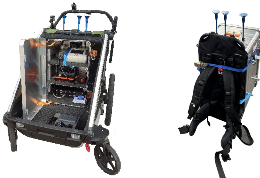
80 81 82 Fig. S1: Photo of the stroller (left) and the frame-rucksack (right) arrangement for walking measurements in the 83 subway and used for other mobile aerosol measurements
