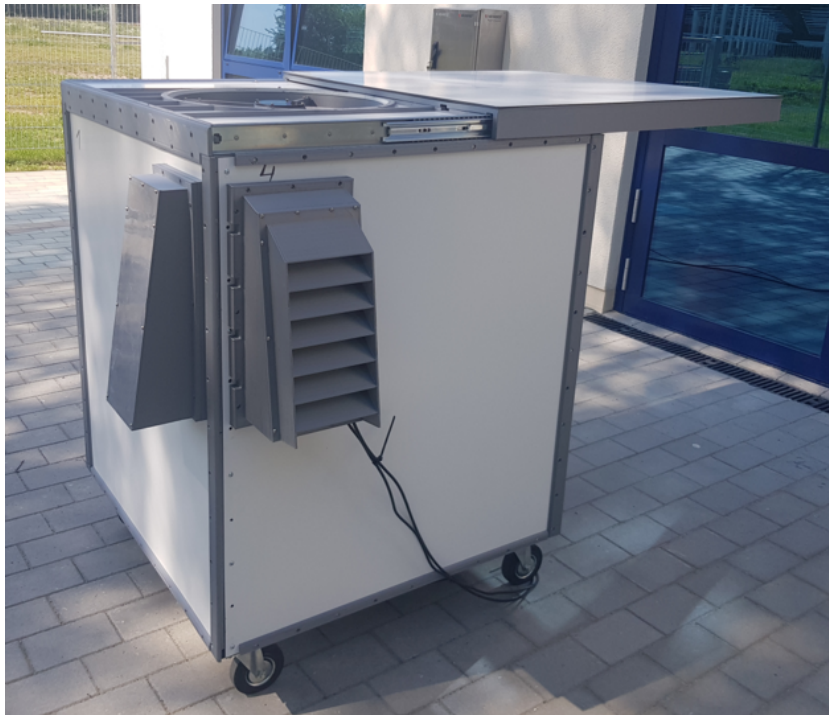
Figure 1.1. Image of the VAHCOLI 0 prototype system during a daylight measurement in 2020 on the test range in Kühlungsborn, Germany. The Prototype system features a small volume of one cubic meter, a weight of 250 kg and is designed for a power usage of 500 W. It uses a single 50 cm telescope and is thus limited to vertical measurements. On the front left edge of the system, the passive cooling solution is visible.
