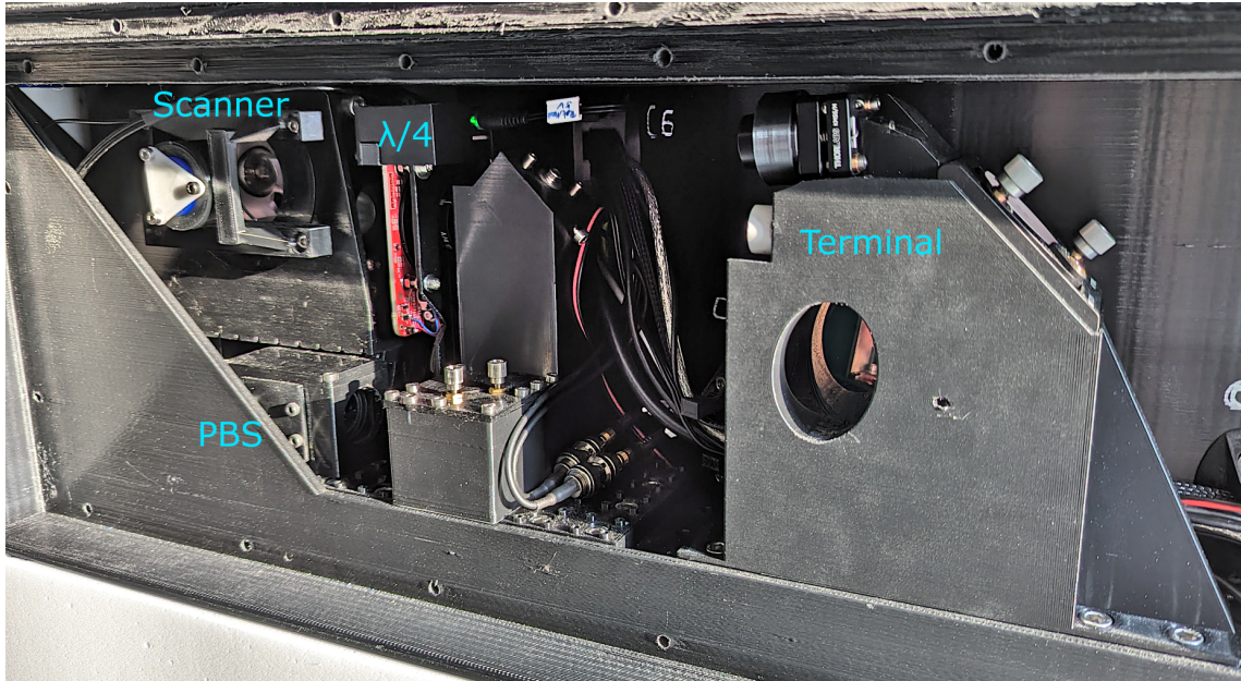
Figure 4.6. Image of the beam switching section as implemented in the VAHCOLI 1 & 2 units. The beam enters the section through the PBS is then diverted upward through the motorised \lambda/4 plate and into the scanner. The scanner steers the beam via an elliptical 1-inch mirror onto the different positions of the distribution terminal.
