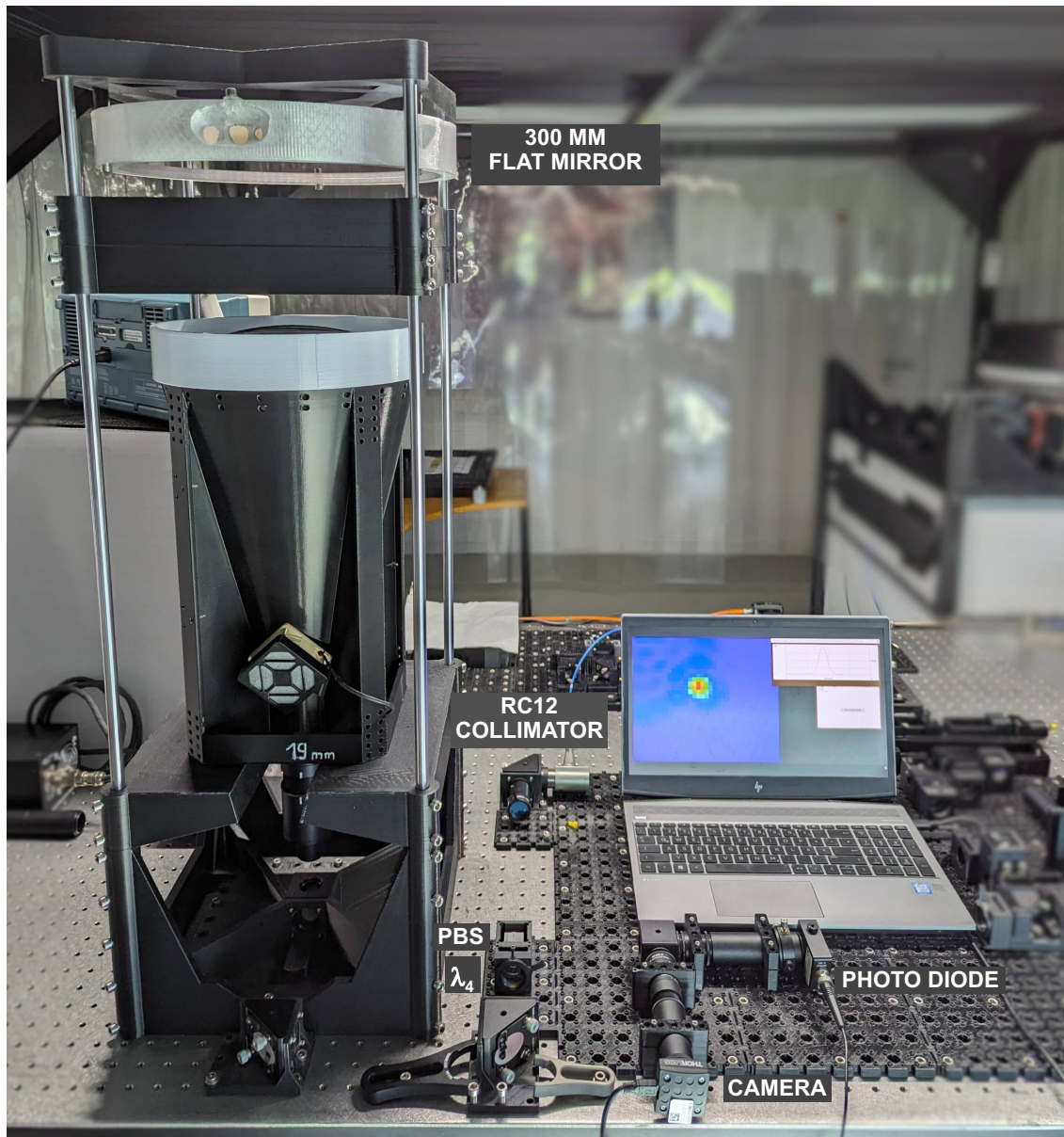
Figure A.2. Image of the autocollimation setup on the optical bench, with one of the lens telescopes for the multi field of view upgrade installed. The 300 mm flat mirror is mounted in a 3D-printed holder, which allows for adjustment of the mirror's angle.
