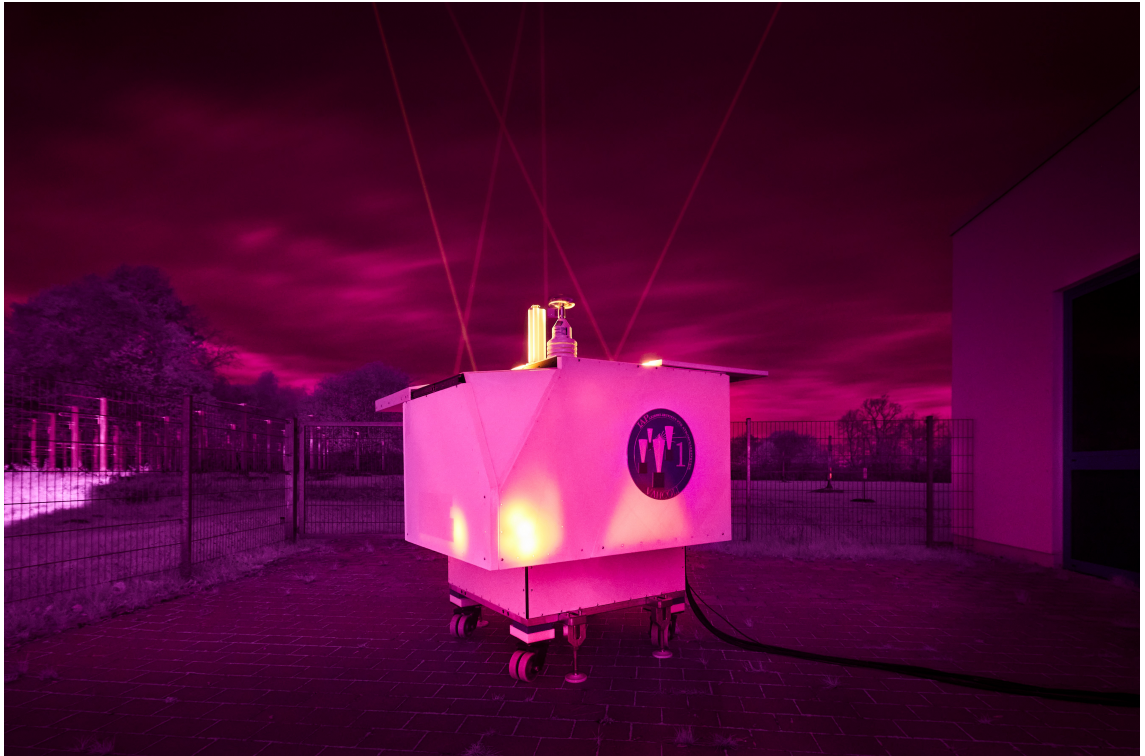
Figure 4.12. Full spectrum photograph of the VAHCOLI 1 unit with the mounted MultiFOV upgrade in operation. © Fraunhofer ILT, Aachen / Ralf Baumgarten“
