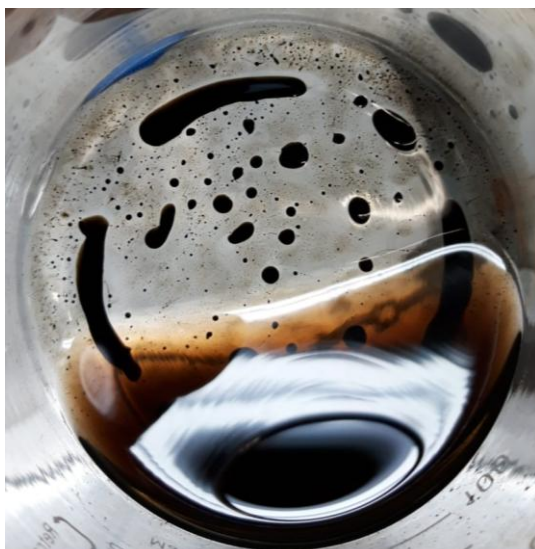
A-28: Reaction product after HDO with guaiacol at 350 °C and 50 bar H 2 pressure.
