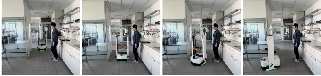
Figure 63 Actual Process of Dynamic Obstacle Avoidance
