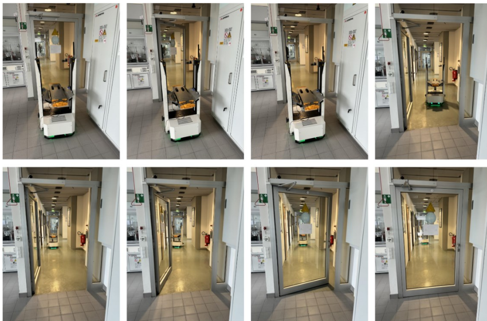
Figure 68 MOLAR Robot Cross Automatic Door
