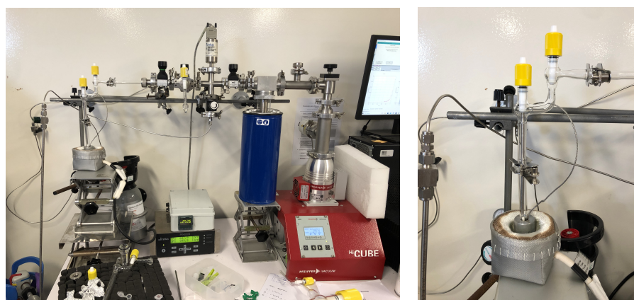
Figure 5.1: Specialized vacuum line providing the possibility to seal a rotor under protective atmosphere. Left: Full line; Right: Rotor containing compartment.
