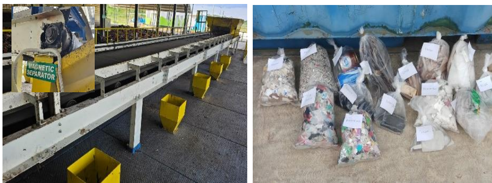
Figure 5.9 Belt Conveyor for Hand-Sorting and Samples for Laboratory Analysis
