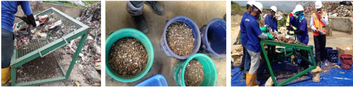
Figure 5. 7 Example of Particle Size Distribution Analysis Processes
