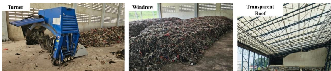
Figure 5. 13 Bio-drying with Turner
