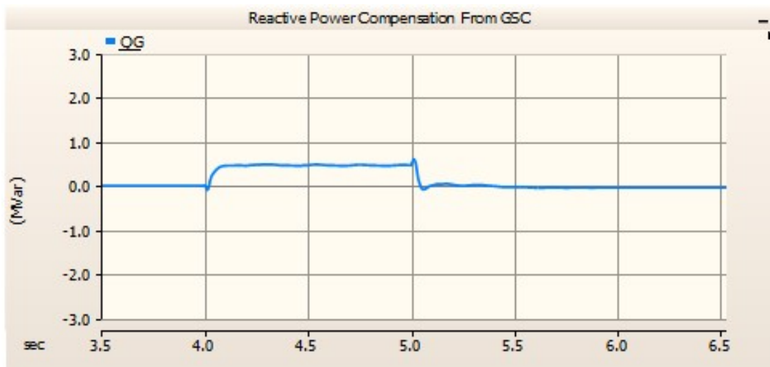
Figure 6.8: Reactive power compensation through GSC for weak grid SCR=3
