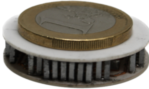
Figure 60: TEG-3 with a diameter of 30 mm, featuring 62 thermolegs with dimensions of 1 \times 1 \times 4 mm 3 . Reprinted from [118].
