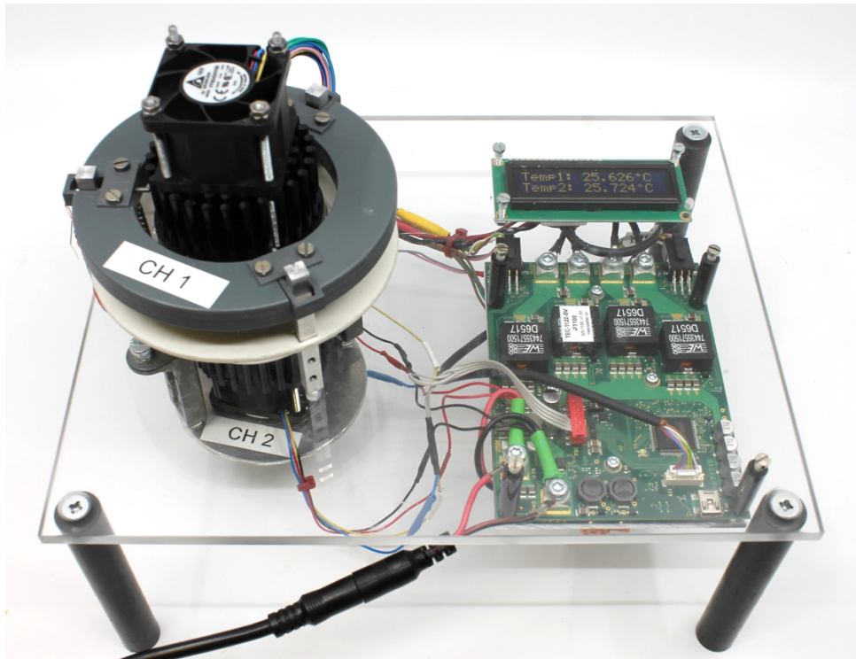
Figure 64: Experimental setup for temperature control during TEG characterization.
