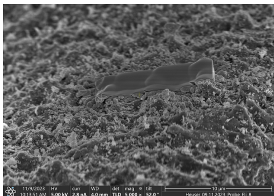
(c) Side view of the ROI coated with platinum.
