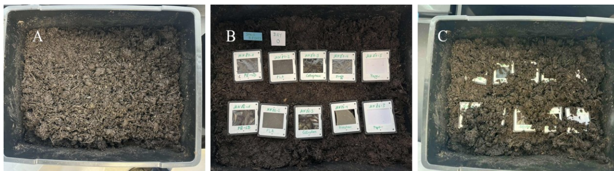
Figure 82. Degradation study in the soil environment. A) the soil box, B) the samples are placed on the soil bed, C) soil buried.
