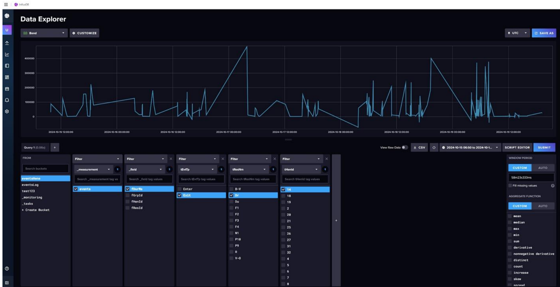
Supplemental Material A: Screenshot of the query interface in InfluxDB's UI Data Explorer, showcasing a real-time time series visualization of RFID event data. The example displays visit durations for a single hen and a specific resource, with options to filter by RFID tag ID and timestamp range, based on automatically detected entry and exit events.
