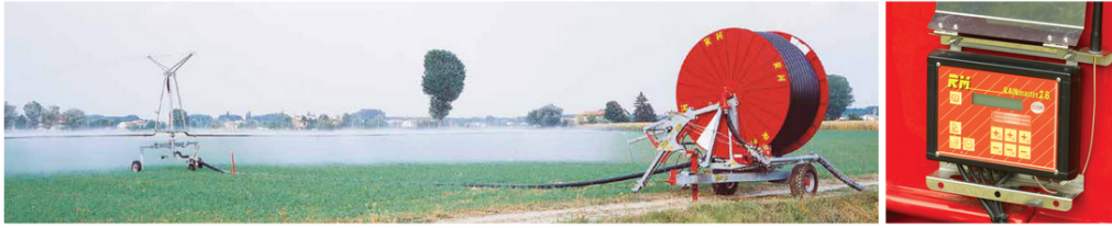
FIGURE 2.2: Hose reel irrigation system with boom configuration (left), with manually programmable speed control unit (right) from the manufacturer RM. Source: RM Irrigation (2025).
