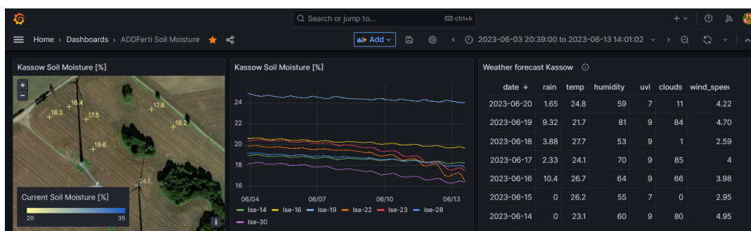
FIGURE 4.4: Grafana dashboard for the Kassow test field in Germany, displaying sensor locations (left), soil MC time series for each sensor (center), and the local weather forecast (right).
