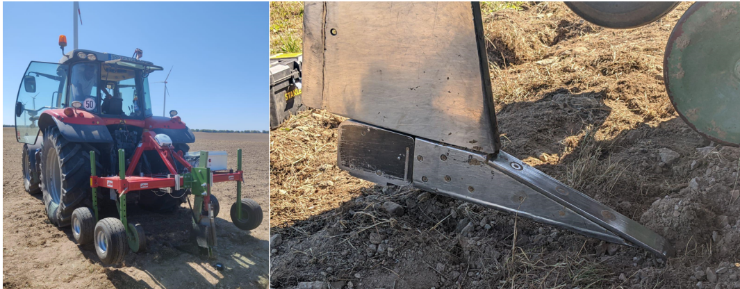
FIGURE 4.8: The on-line vis-NIR multi-sensor platform developed by Mouazen and Ramon (2006) on the field in Kassow, Germany in August 2022 (left). The vis-NIR sensor is located on the heel of the subsoiler (right).
