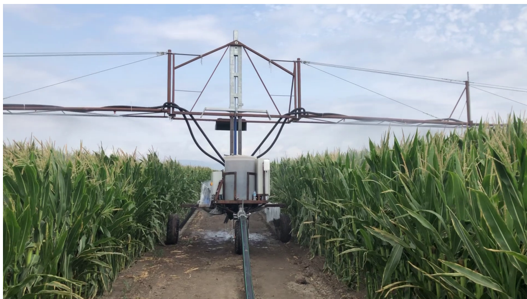
FIGURE 7.9: Boom of the HIS during the field trial in Field 3, Turkey, on 24 August 2023, showing the mounted 300 L fertilizer tank and the supply lines for the four boom sections.
