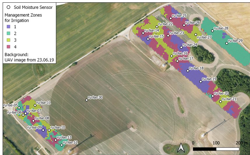
FIGURE 4.5: Locations of LoRaWAN soil moisture sensors in the Kassow test field, Germany, shown in relation to the delineated irrigation MZ.
