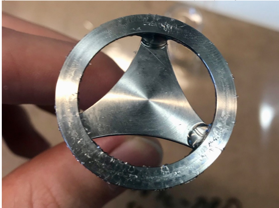
Figure 65: Thermo Scientific titanium ring-rotor with gelled particles after 24 h measurement.
