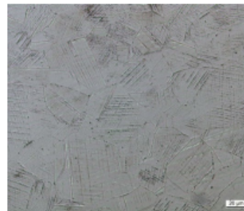
Figure 4. The microstructure of X2CrMnNiN17-7-5 in the deformed area of a transverse bend test sample at room temperature (left) and at -80°C (right)
