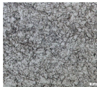
Figure 5. The microstructure of 9% Ni steel in the deformed area of a transverse bend test sample at room temperature (left) and at -80°C (right)
