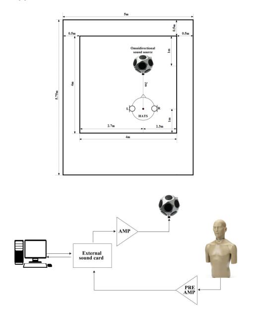
Room:Audio Laboratory University of Rostock (Germany)Size:  $5.75 \,\mathrm{m} \times 5.0 \,\mathrm{m} \times 3.0 \,\mathrm{m}$ acoustically treated, low reverberation time  $T_{60} \approx 0.3 \,\mathrm{s}$
