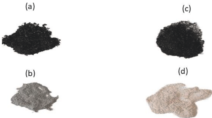
Fig. 1: Rice husk after heating for volatile matter and ash content (a) single-stage sample (after heating for the volatile matter), (b) single-stage ash content, (c) double-stage sample (after heating for the volatile matter), (d) double-stage ash content
