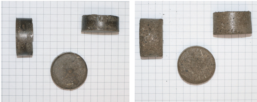
Abb. 4: Briketts aus 100 Ma.-% Gärrest (Charge BGA CBC 2), links Brikettcharge 1, rechts Brikettcharge 5
