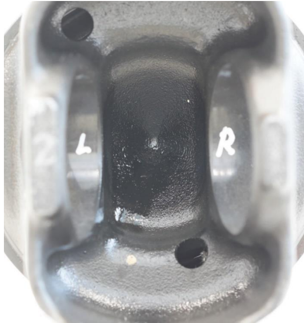
Figure 17b: Piston bottom of cylinder 1
