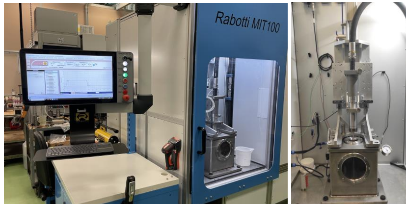
Figure 3: PFI injector test bench (left), detailed view of the injection chamber (right)
