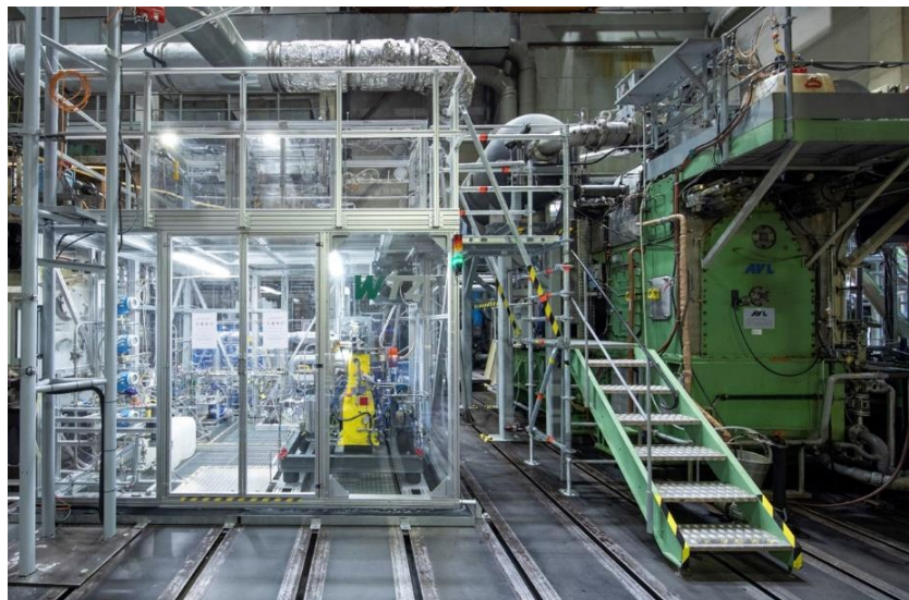
Figure 4: Methanol conditioning unit (left) and the MAN-32/44DF-M SCE Engine test bench (right) at WTZ, Roßlau
