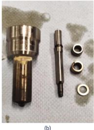
Figure 10: (a) Nozzle tip after testing; (b) Nozzle, needle, inner parts: all clean using a proper working blend
