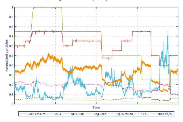
Figure 8: Test run with a problematic bio-oil blend
