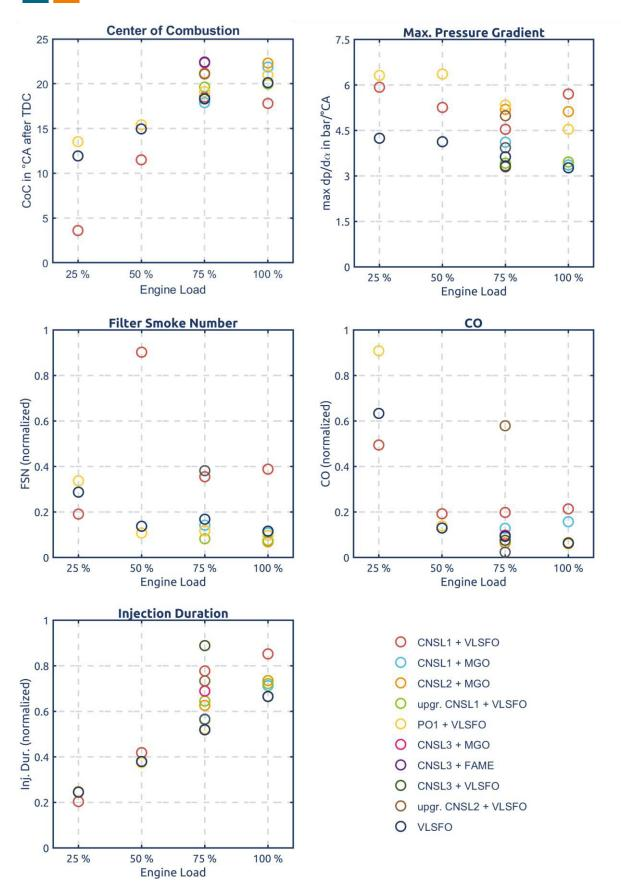
Figure 9: Comparison of engine parameters for different bio blends
