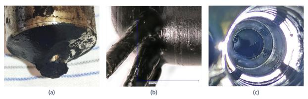
Figure 12: (a) Massive coking on nozzle tip; (b) Still good state of nozzle interior; (c) Large deposits on the underside of the cylinder head in all cylinders
