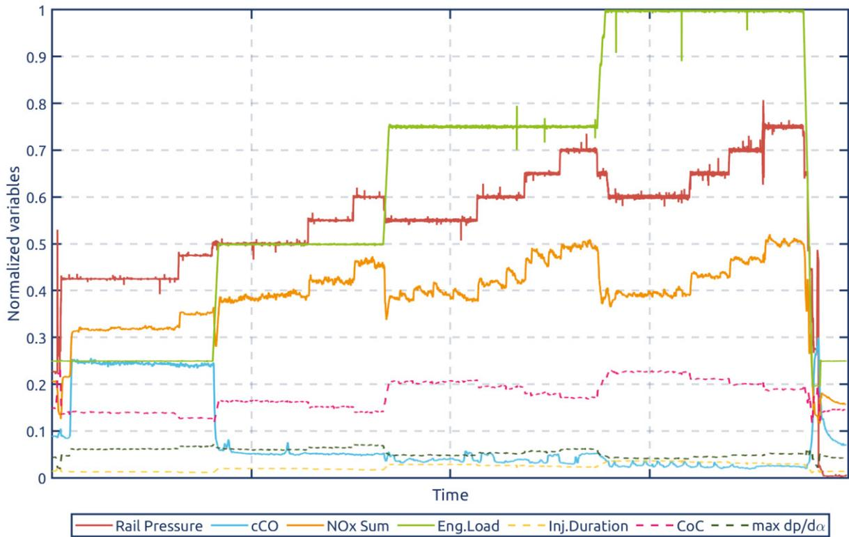
Figure 7: Test run with a promising bio-oil blend
