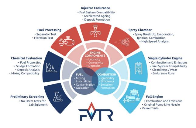
Figure 4: Compatibility issues and testing methodology for bio-oils and blends
