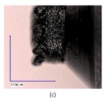
Figure 11: Nozzle imprints after test run with (a) Reference VLSFO, (b) a suitable bio blend and (c) a bio blend hard to operate
