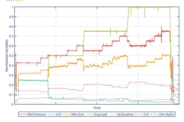
Figure 7: Test run with a promising bio-oil blend
