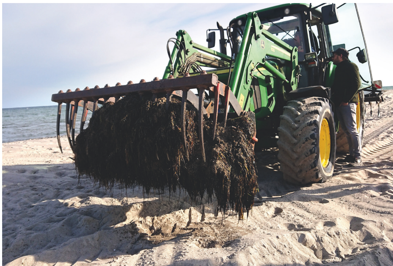
Figure 31 Mechanical collection of beach wrack (© J.Hofmann)
