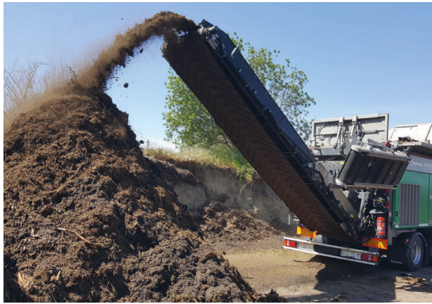
Figure: 1.16 Shredding and mixing of green waste and beach wrack
