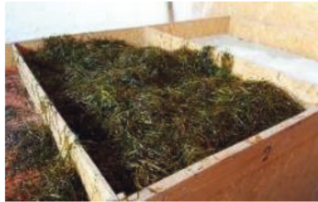
Figure 1.10 Active drying with a fan and an electrical heater in wooden drying boxes at the Hanseatische Umwelt CAM GmbH facilities, July 2020)
