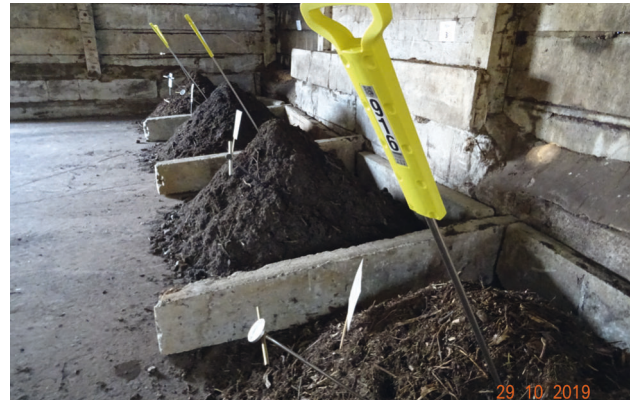
Figure 1.14 Compost piles with wireless temperature probes at the Hanseatische Umwelt facilities, October 2019
