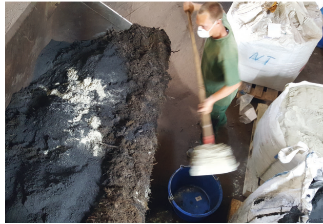
Figure 1.17 Adding additives to the compost
