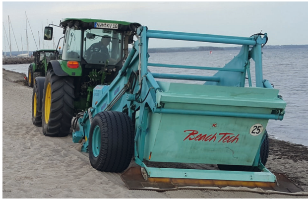
Figure 1.4 Collection with a tractor and a beach cleaning vehicle "Beach Tech STR 2000" (Island of Poel, Germany, July 2020)
