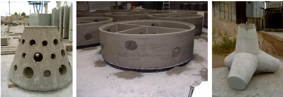
Abb. 5: Betonelemente – links: Riffkegel, Mitte: Ring, rechts: Tetrapode.
