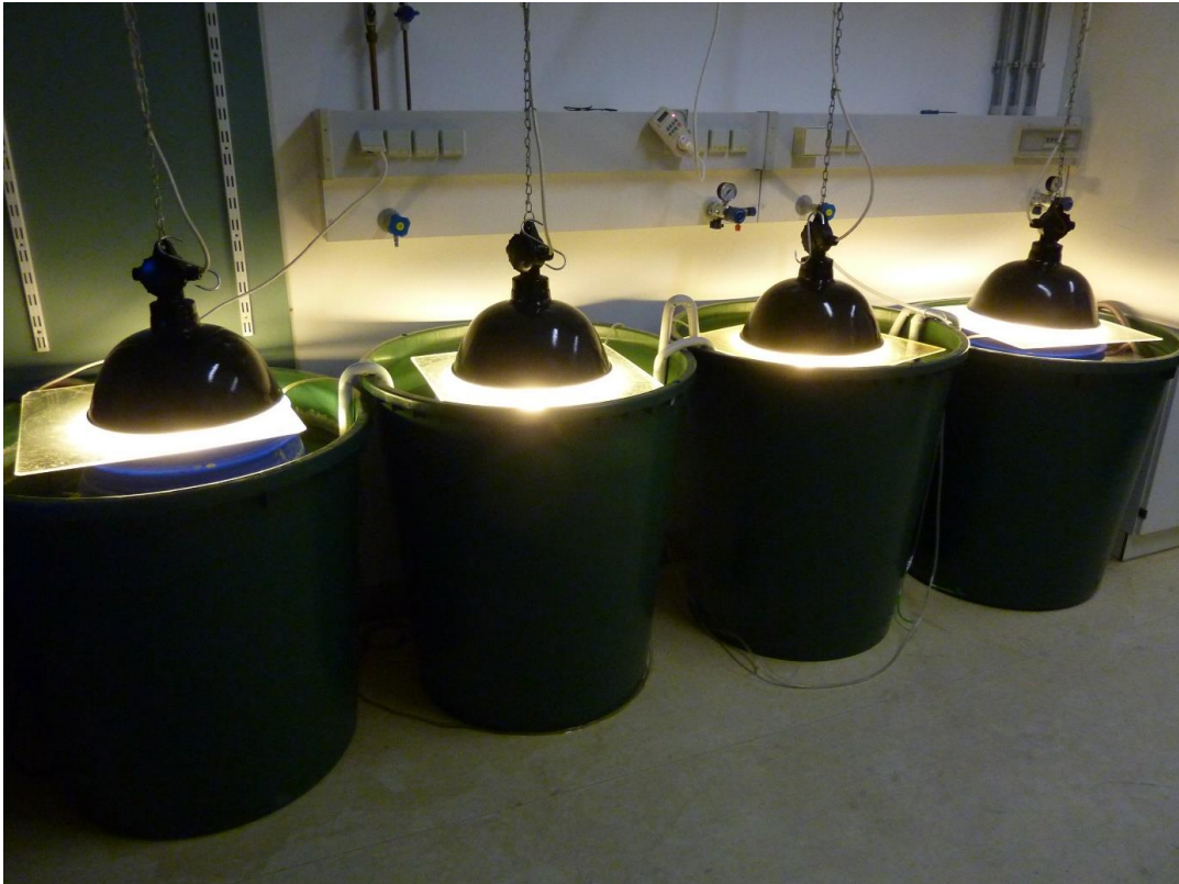
Fig. 1: Mesocosms setup with 4 replicates, each mesocosm (blue barrel) is surrounded by a water jacket (green barrel), which are interconnected by tubes and a pump.
