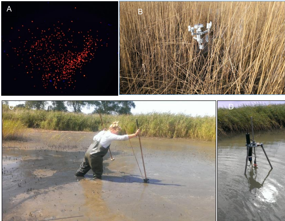
Fig.2: (A) Fluorescent tracer particles under UV light (only tracer particles without “normal” sediment particles) (B) Wireless weather station inside reed stands to measure wind attenuation. (C) Usage of the stamp sampling device with grease-coated cards in a muddy area of the basin. (D) The 3D acoustic Doppler velocimeter ( Vector – Nortek ) measures three velocity components (X, Y, Z) based on an acoustic echo from particles.
