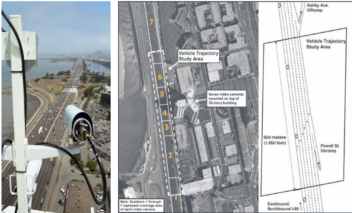
Figure 2.1.: The aerial photograph of the I-80 study area in relation to the building from which the video cameras were mounted and the coverage area for each of the seven video cameras. The pictures taken from [2].
