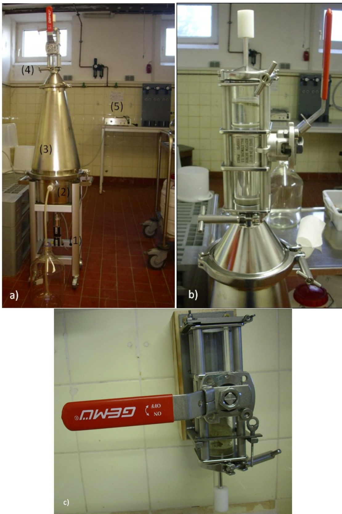
Figure 5: Munich Plastic Sediment Separator (MPSS) built by Hydro-Bios setup (a): motor (1), sediment container (2), stand pipe (3), small cone and dividing chamber (4), controller (5); ideal filling level in the upper sight glass (b); dividing chamber in the mounting with the ball valve closed (c)
